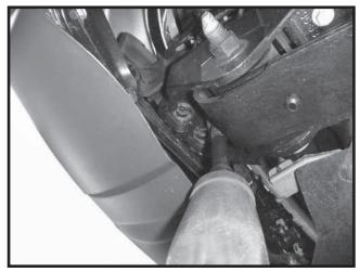
2. Pull bumper forward and remove three tow hook bolts. The tow hook or bolts will not be reused.
